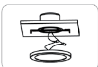
② Connecting the wire.
